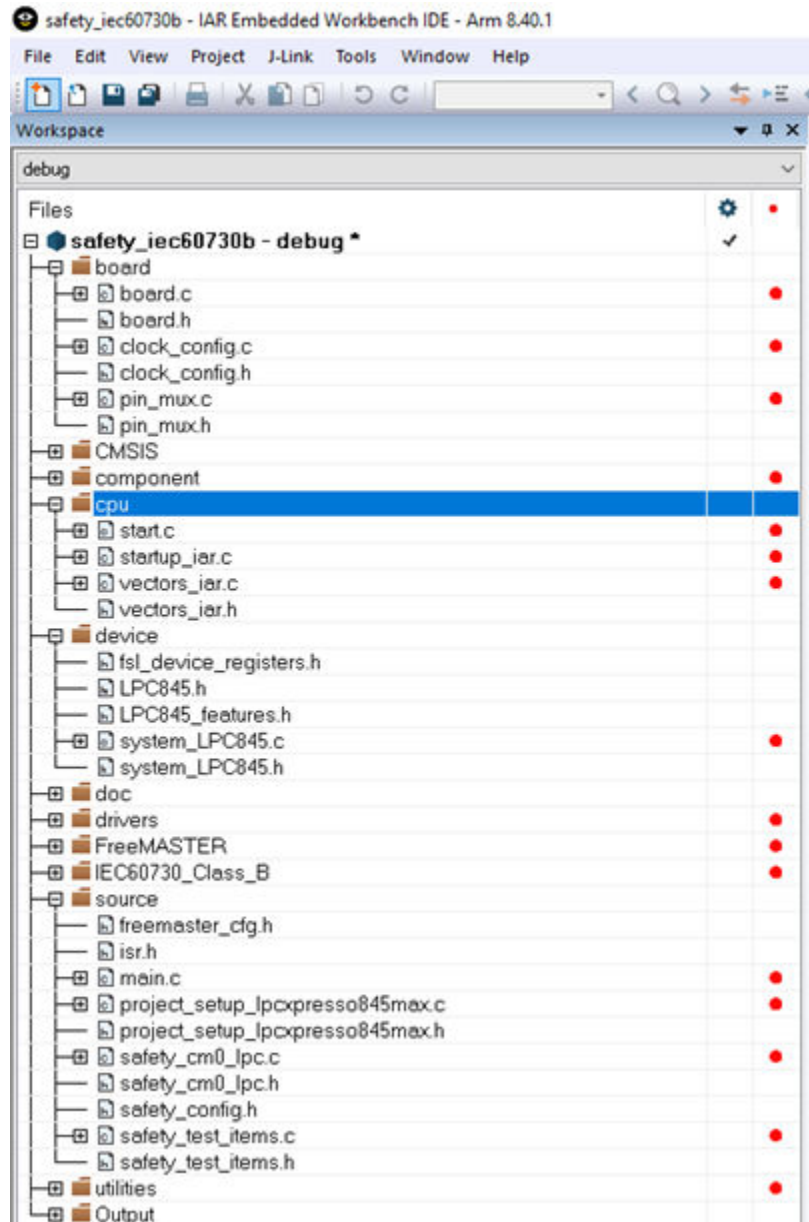
Figure 5. IAR example application structure
