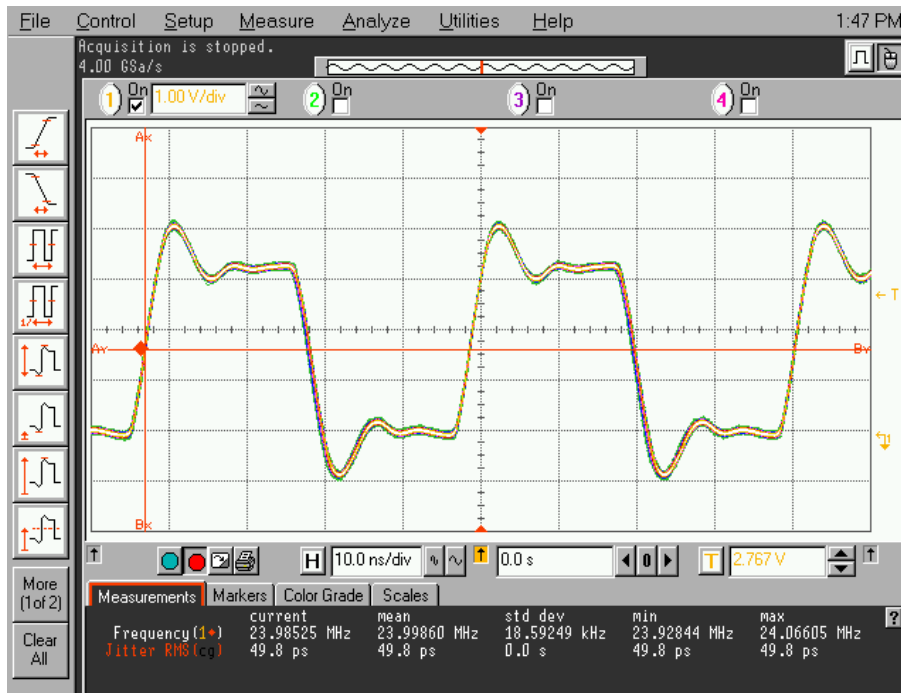
Figure 12. RMS jitter of single-ended 24.000 MHz CLK02 (A17 ball) output of SABRE-AI design (i.MX 6Solo, OBDS)
