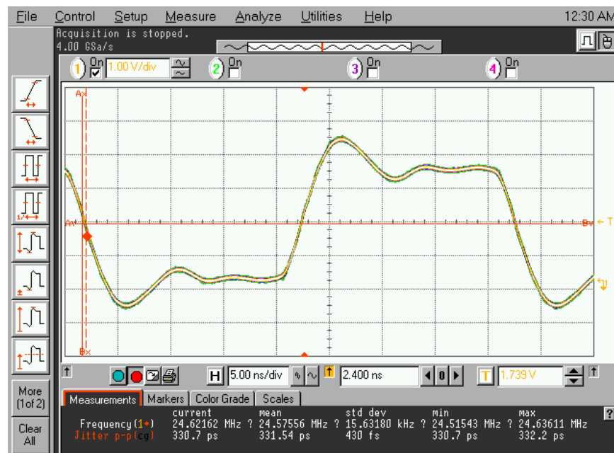
Figure 5. Peak-to-peak jitter on external oscillator single-ended 24.576 MHz output of SABRE-AI design (i.MX 6Solo, OBDS)
