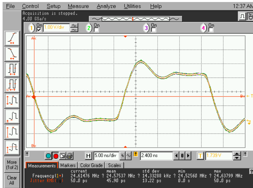
Figure 4. RMS jitter on external oscillator single-ended 24.576 MHz output of SABRE-AI design (i.MX 6Solo, OBDS)
